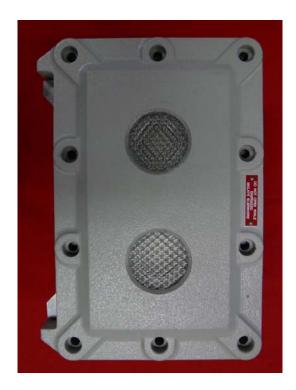
FJB210WL2 front view. The green and red light sources are solid-state and designed to last for life. The reflectors are internal, therefore are protected from dust and weather. The diffusers can be replaced from outside.
